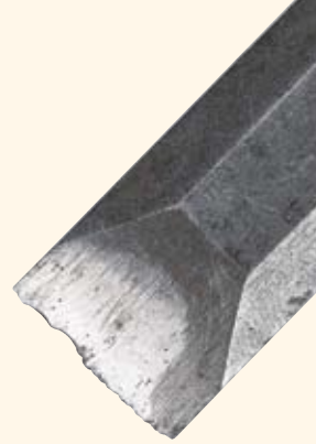
▲ This edge is badly nicked and the bevel is too shallow.
